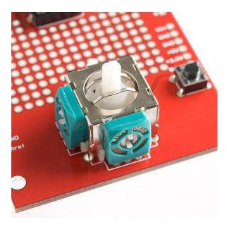
Once you've applied enough pressure to the top of the joystick case all the legs should poke through the bottom of the PCB—the structural legs will protrude further than the others:
