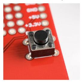
Next turn the board over and you should see those cute little legs pointing through the holes in the PCB. If they don't extend as far as shown in this picture check you have the orientation correct and then apply a little more pressure to pop the legs through. The button shouldn't fall out of the holes when you turn the PCB upside down.
