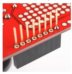
Then we solder the pin at the opposite end of the header and re-check the alignment:
