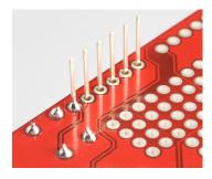
The reason we start with just one pin is because it makes it easier to obtain the correct alignment and fix any mistakes. Once you've soldered one pin you might want to test the alignment by inserting the shield into an Arduino. Just be careful when you do so because the header's still only held in place with one solder
