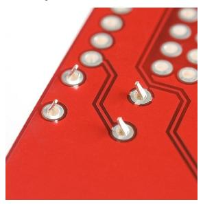
Now it's time to solder the first leg—it doesn't matter which of the four you start with—but ensure the plastic bottom of the button is still flat against the PCB. Apply heat with the soldering iron simultaneously to the leg of the button and the pad (the circle of track around the hole) on the PCB then carefully feed a little piece of the solder into the joint formed between the soldering iron, pad and component leg. Then remove the solder wire and then the soldering iron—in that order.
