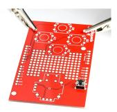
You can see more clearly below that the legs splay out slightly. There's two pairs of legs on opposite sides of the body—one pair should sit in the set of holes close to the edge of the PCB while the other pair should sit on the opposite short-edge side of the white rectangle marked ("silk screened") on the PCB.
