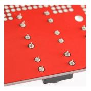
Once again it's time to solder the first of the button legs. My suggestion is to start with the button closest to the middle of the board and work left to right and down from there so you don't have to move the soldering iron over already soldered joints. Again the order isn't critical though.
