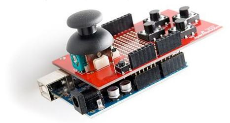
Once you're happy with the alignment of the header you can solder another pin into place—my recommendation is to solder the pin at the opposite end of the header to the first pin you soldered. The reason for this is that once the two end pins are in place the alignment won't change. I recommend double checking the alignment is still okay again by connecting it to your Arduino again.
