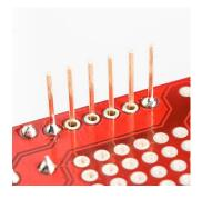
After you've confirmed the alignment you can solder the remaining four pins into place:
