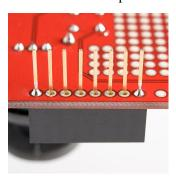
And finally we solder the remainder of the pins in the middle of the header.
