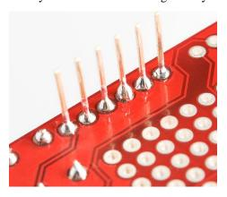
At this stage you can repeat these instructions for the second 6 pin header or skip ahead to solder the diagonally opposite 8 pin header. Soldering a 8 pin header now helps to get the alignment right.
