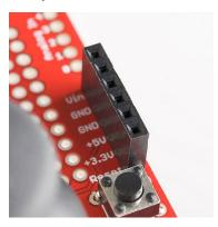
If you don't have a PCB vise then you will probably want to temporarily put one of the 8 pin headers into its location so that the PCB is level when you solder the headers. The headers won't stay in place when you flip the board over so hold them in place when you turn the PCB over to leave the pins sticking
