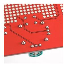
If you've already attached the headers you can now flip the board over and reattach the plastic hat to the white center post of the joystick—take note that it will only fit in two orientations as the center post is rectangular. You can now skip to the <u>Completed Soldering section</u>.
