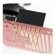
Next solder one of the pins into place. Ensure the header is aligned as parallel as possible to the edge of the board when you do this:
